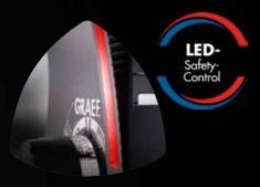
Most accidents happen after slicing that's why the unique GRAEF safety concept on the SKS 700 provides a constant reminder of the open stop. The blue light signals that the slicer is ready for use. After a minute, the light turns red and then starts to pulse after a further 240 seconds – until the stop is closed. 100% innovation for 100% safety.
